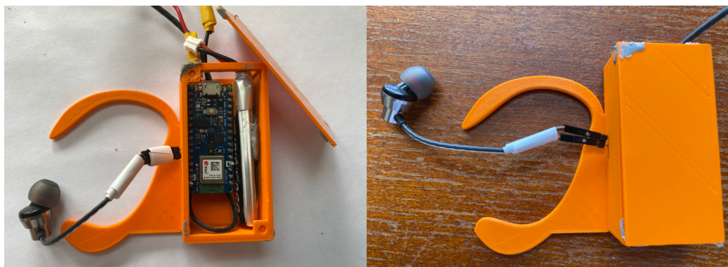
Fig. 1.2: Final earable prototype
