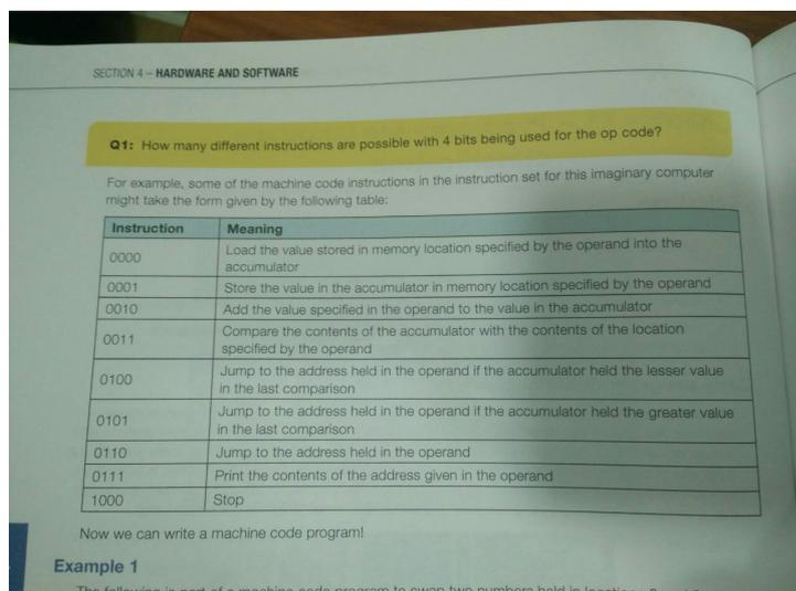
The above table shows the possible opcodes of lots of different commands. Machine Code is a very low-level programming language, because the code reflects how the computer carries out the command – it is dependent on the specific architecture of the computer.
