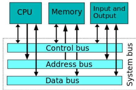
**I/O Controller:** The IO Controller is a device which interfaces between an input or output device and processor. Each device has a separate controller which connects to the control bus. IO Controllers receive input and output requests from the processor and then can send signals to the device they control. They also manage the data flow to and from the device. The controller is made up of three main parts:
